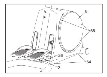
Remove the right Pedal Bracket (13) by removing the two M10 x 82mm Button Bolts (26) and the two M10 Nylon Locknuts (not shown). Then, remove the two M4 x 38mm Screws (64) and the three M4 x 25mm Screws (65). Carefully slide the Right Side Shield (8) off the stepper.
